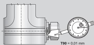
Maximum runout of output spindle
